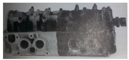
Figure 8.5: Half of the cylinder head was cleaned with a soda blaster
